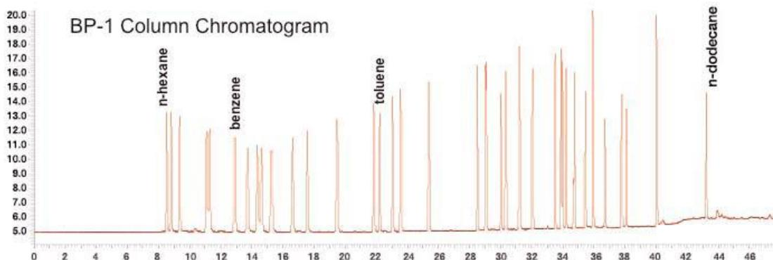
PAMS use thermal desorbers equipped with cold traps to analyze ozone precursors which are either too volatile or too labile to be sampled/stored by a primary sorbent tube. The chromatograms above (courtesy of PerkinElmer, Inc.) show the dual-column separation of a 2-ppb standard of ozone-precursor target compounds
